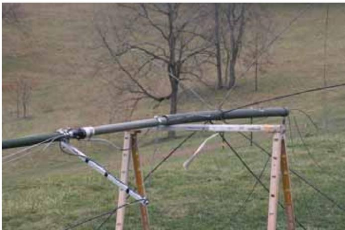
Photo 2 (left) shows the very top of the antenna. The last few feet are paired #10 conductors, going up to a "spider" which is the top load. Even though this assembly is light weight fiberglass, it does make the antenna top heavy, which is part of why I want to truss it to make it more rigid.
