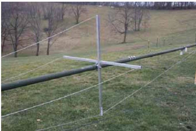
matched, I often saw the tuner retune during a transmission reacting to changes in impedance as the antenna moved around. This was hard on the tuner and imposed an additional form of modulation on the transmitted signal. I dealt with this by constructing a control panel which let me lock the tuner, once initial tuning was accomplished. The black wire at the bottom of the photo is the #8 shunt feed conductor, which is at a 45-degree angle to the truss spreaders that surround it.
