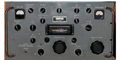
Collins R-390 receiver, the "work horse tool of the CT", used in the 1970's for monitoring. Photo courtesy of & © 2017 Dan Flanagan W3DF ex GM5ASI
