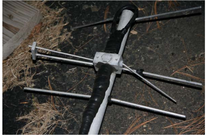
Destroyed driven element assembly. Note the machined connection area which allows for rigorous waterproofing of balun and feed
