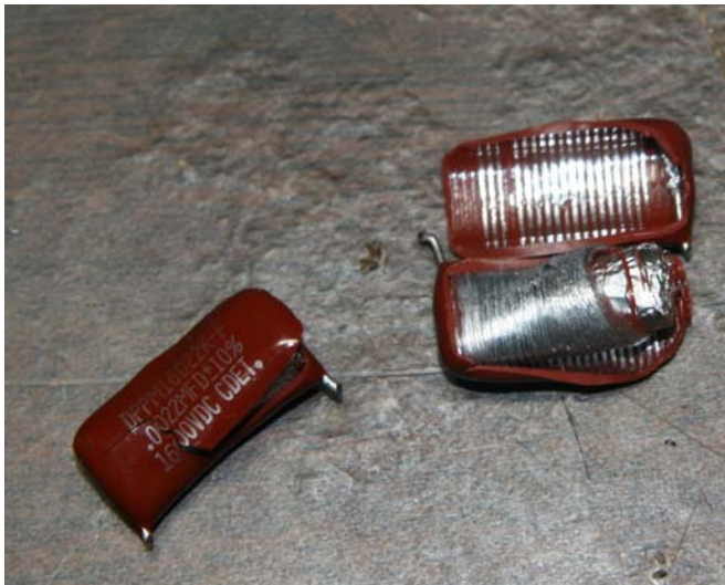
Blown caps from the N3SH 40 Meter bandpass filter. Complete article on the filters can be found on the N3SH.ORG web site
