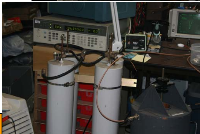
The 2 M bandpass filter & the results (on the analyzer, top right)
