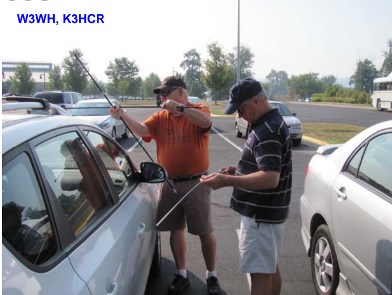
Above & Below: Assembling the 40 Meter Hamstick Dipole on Larry's Car , raising it on his trailer hitch
