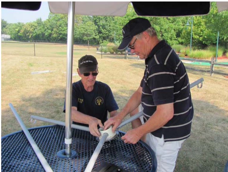
Below: K3VX & K3HCR assembling the 20 meter hamstick dipole support "structure" out of pre-cut PVC
