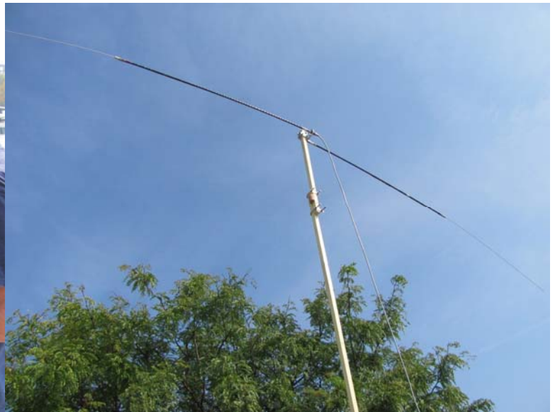
Below: K3VX & K3HCR assembling the 20 meter hamstick dipole support "structure" out of pre-cut PVC
