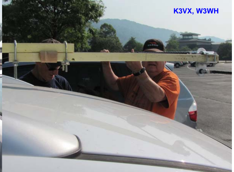
Above & Below: Assembling the 40 Meter Hamstick Dipole on Larry's Car , raising it on his trailer hitch
