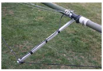
matched, I often saw the tuner retune during a transmission reacting to changes in impedance as the antenna moved around. This was hard on the tuner and imposed an additional form of modulation on the transmitted signal. I dealt with this by constructing a control panel which let me lock the tuner, once initial tuning was accomplished. The black wire at the bottom of the photo is the #8 shunt feed conductor, which is at a 45-degree angle to the truss spreaders that surround it.
