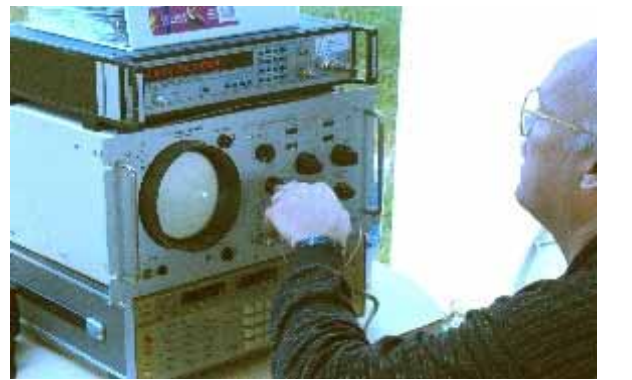
Above & Below: WB4GCS Vector Analyzer
