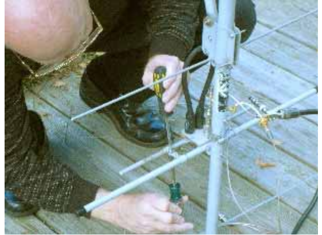
Adjusting the 222 MHz Beta Match
