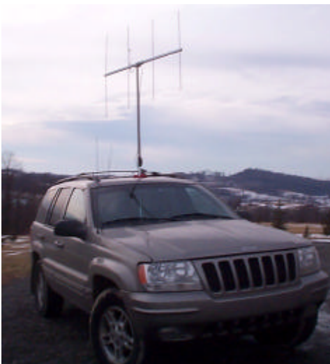
I used a 4 element, beam (Arrow brand) on a 6 foot mast, through the sunroof. Retracted slightly as I traveled to my three locations: Bridgeville, Scott Twp, and Mt. Lebanon. Power out: 10 watts. — KE3XB
