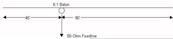
The OCFD is a simple coax-fed wire dipole antenna that is often incorrectly referred to as a Windom. It measures 135' in overall length, and works best in a flattop configuration, or the ends can be drooped toward the ground to fit a particularly small lot. In fact, if installed 25' high, BOTH ends could be drooped 10' and still keep things safely 15' up while only taking up the space needed for a G5RV. And anyone who has ever fooled with a G5RV knows they can be a real BEAR to tune at times!
